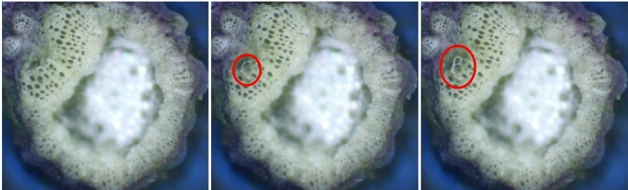
Figure 2: Visual endpoint indication: The left picture shows the petiole without efflux about 2s before the endpoint was determined, the middle picture displays the moment the endpoint got indicated, the right picture shows the increase in efflux directly after the endpoint's indication (< 1s).
