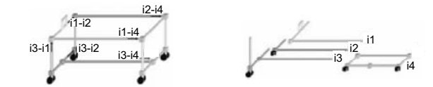
(e) Inner frame of the structure (f) Components of the inner frame
