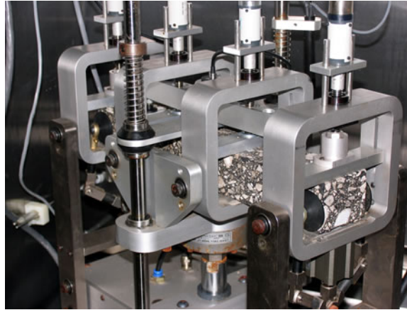
Figure 2.2: 4PB test configuration.
