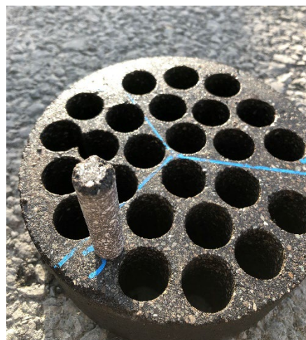
(b) A FAM specimen cored from the cylinder
