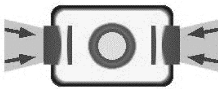
Figure 1.1: An idealized ICF hohlraum; Arrows indicate application of driver energy
