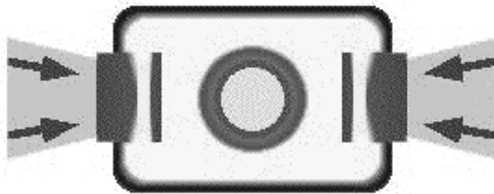
Figure 1.1: An idealized ICF hohlraum; Arrows indicate application of driver energy
