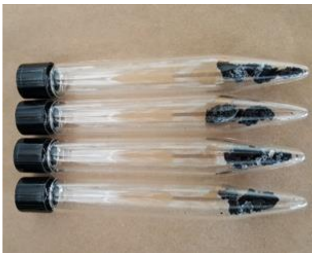
Figure 26: Glass centrifuge tubes containing the \text{TiB}_2 synthesis products prior to washing with deionized water and 2M HCl.
