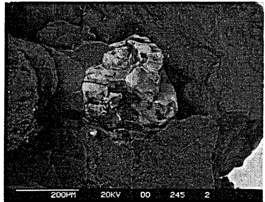
Fig. 23 Roosevelt Hot Springs Tuff (Thermal Power). Accessory Magnetite (Backscatter Detector)
