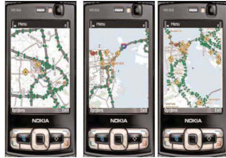
Mobile Millennium traffic client. Traffic is displayed directly on the phone screen, with traffic information such as construction, accidents, etc., and audio traffic reports. For drivers who want to opt in, the phone can also send information to the system (Lagrangian measurements).
