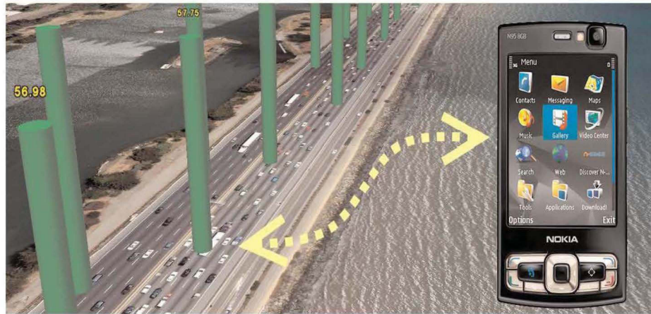
Fig. 1. The Nokia N95 mobile device is used to collect and transmit anonymous speed and position data when on-board vehicles. The height of the columns correspond to the speed of a vehicle equipped with an N95 on I-80 near Berkeley, CA.
