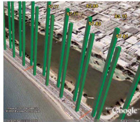
A Google Earth rendering of collected GPS data. Virtual trip lines measuring speed upon crossing of the vehicles are shown in red.
