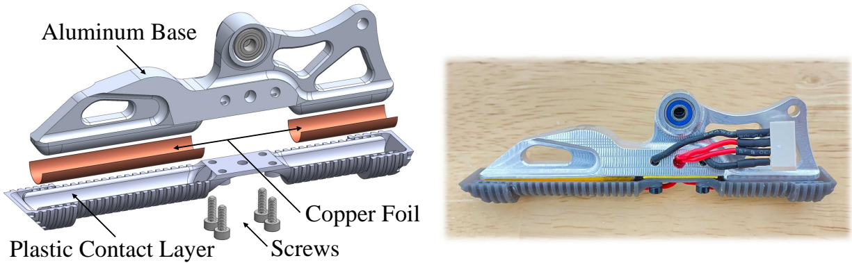
Figure 2.5: BRUCE contact sensing foot V1. On the left is the exploded view of the CAD model and on the right is the hardware assembly. For the assembly, the two copper foils are glued to the plastic contact layer, which is then attached to the aluminum base using screws.
