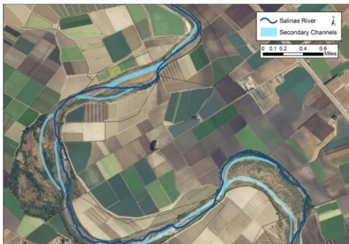
Figure 6. Proposed secondary channels in a section of the Salinas Rivers. Secondary channels are typically 0.25-0.75 miles long and connect with the main stem of the river at their upstream and downstream ends (RCDMC 2020).
