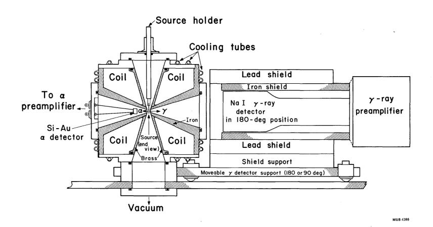
Fig. 1. Diagram of the angular correlation magnet.
