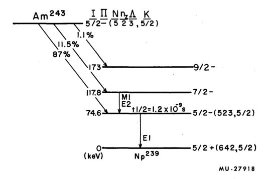
Fig. 2. Partial decay scheme of Am<sup>243</sup>. This figure was taken from reference 1.
