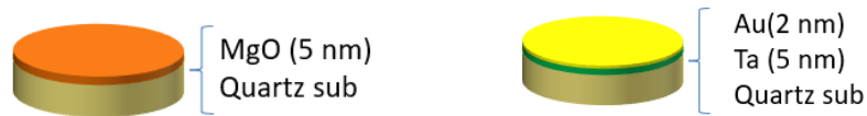
Figure 4.6 Multilayer structure of fabricated samples used for optical thin-film measurement of MgO and Ta.
