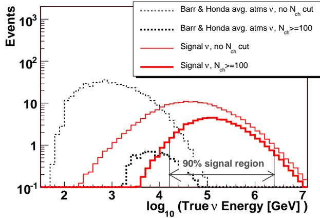
FIG. 5: The true energy of the simulation is shown for atmospheric neutrino and signal events. The thin dashed (atms.  $\nu$ ) and solid (signal  $\nu$ ) curves represent the number of events before the  $N_{\text{ch}} \geq 100$  requirement. The thick dashed and solid lines represent only the events in the high energy sample.
