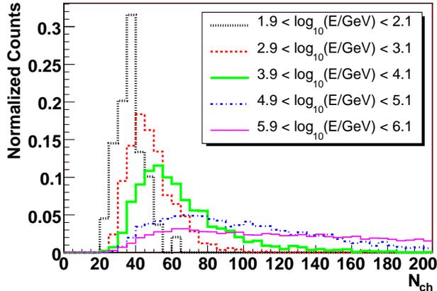
FIG. 2: The number of OMs hit during an event ( $N_{\text{ch}}$ ) was used as an energy-correlated observable. Each line on this  $N_{\text{ch}}$  distribution represents events with approximately the same simulated energy. High energy events may not be contained within the detector and hence can trigger a wide  $N_{\text{ch}}$  span.
