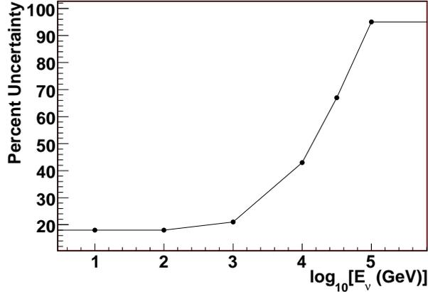
FIG. 12: The estimated uncertainty in the atmospheric neutrino flux as a function of energy. Due to the large uncertainty in the prompt neutrino flux at greater than  $10^4$  GeV, the total uncertainty rises sharply.
