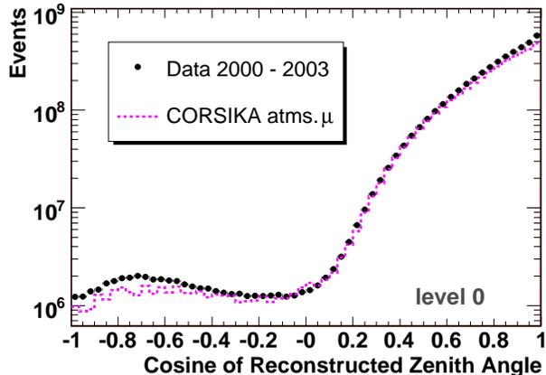
FIG. 1: The cosine of the reconstructed zenith angle is shown for every event at the beginning of the analysis (level 0). The experimental data is dominated by downgoing atmospheric muons. Events reconstructed as upgoing appear on the left side of the plot and downgoing events appear on the right.
