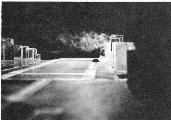
FIG. 9. Smoke tracer showing updraft on face of tallest building. Wind is from the south-east.
