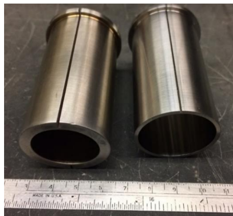
Figure 4.8: Original (left) and enlarged (right) stainless steel burner heads.
