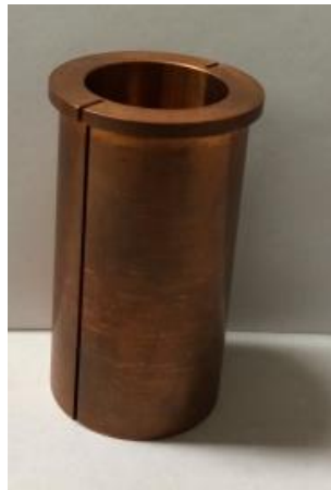
Figure 4.7: Burner head constructed of copper.
