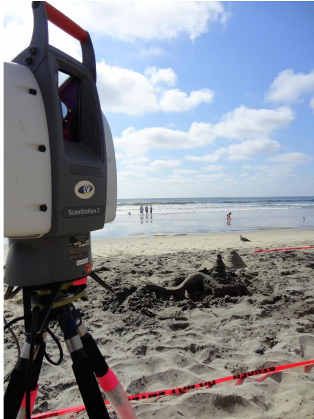
Figure 12: The Leica Scanstation 2 poised to begin the third round of scanning at Torrey Pines Beach.
