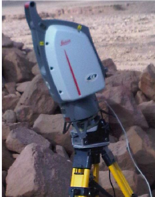
Figure 5: The Tilt Head is displayed in action, poised between a surveying tripod and the tribrach and scanner in the field in Jordan. Image by author.
