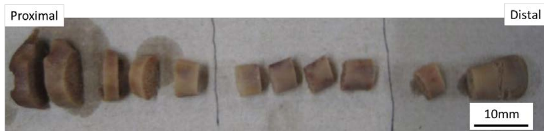
Figure 15: The duck humerus bone after being sectioned into 5mm portions.
