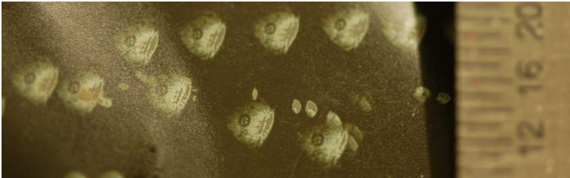
Fig. 3.2 Single shot burn patterns measured on Zap-It burn paper at 486nm mode output from a PDL dye laser with the THG pumped longitudinal pumping. Additional Telescoping Optics were installed in the PDL to narrow the mode diameter to match the mode of the PDL mode output. The Gaussian Output coupler mirror's imprint from a Continuum Surelite, overlap onto the PDL output is observed.
