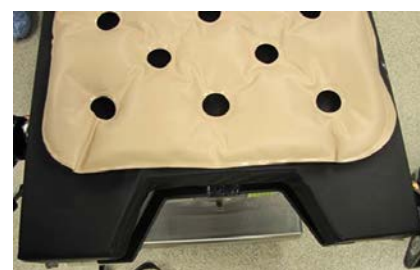
Figure. Photograph of the pressure mapping pad placed atop the operating room table.
