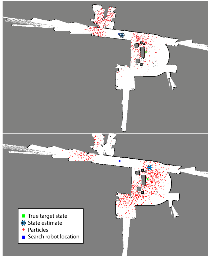
Figure 5.20: Different estimation modes for the PILOT particle filter. MMSE state estimate [top], maximum weight particle estimate [bottom]
