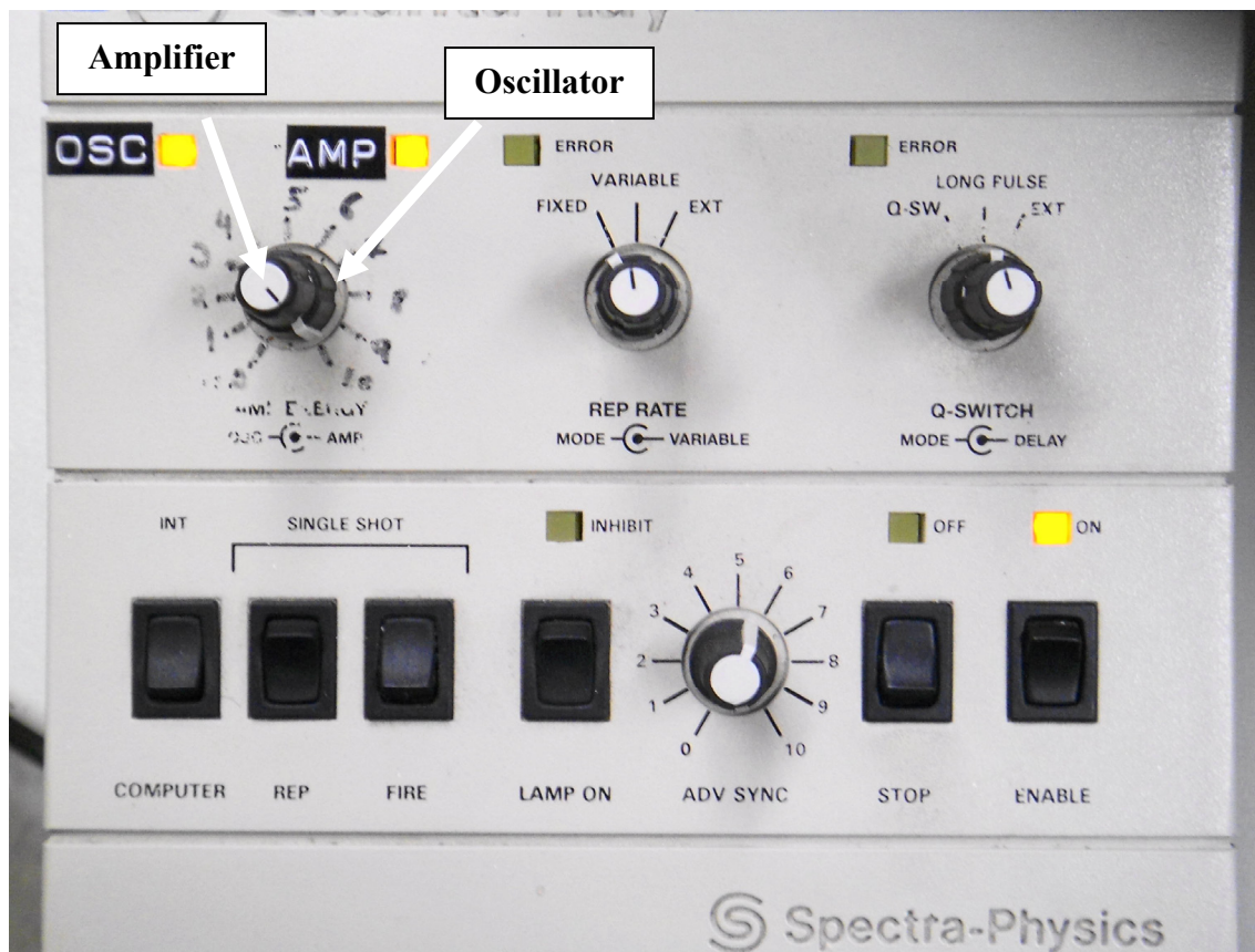
Figure A.3: The GCR-270 YAG controller in LONG PULSE MODE. [File: FA.3]
