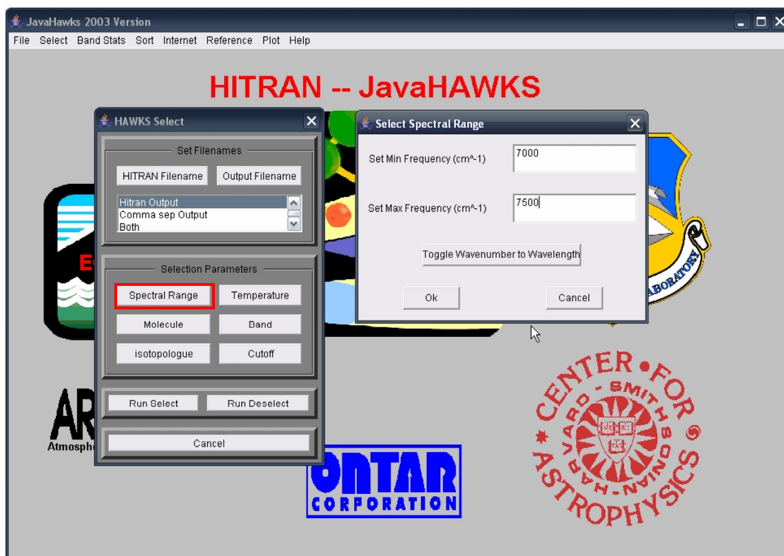
Figure F.21: Computer screen caption of the HITRAN program. Selecting the Spectral Range option prompts the user to set spectral range in \text{cm}^{-1} or \mu\text{m} units. [File FF.21_hitran8]
