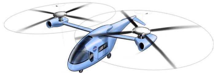
Fig. 1. NASA's six-passenger side-by-side conceptual design [20].
