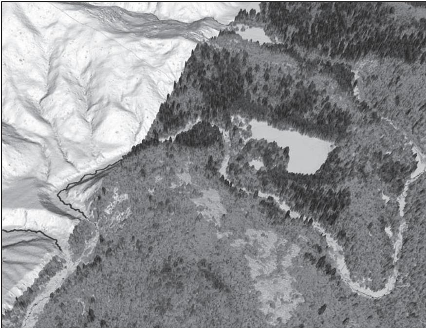
LIDAR'S VIEW OF THE ANGELO RESERVE — A SMALLER SECTION IN GREATER DETAIL — SHOWS INDIVIDUAL TREES. IMAGE COURTESY OF THE NATIONAL CENTER FOR EARTH-SURFACE DYNAMICS (NCED)
