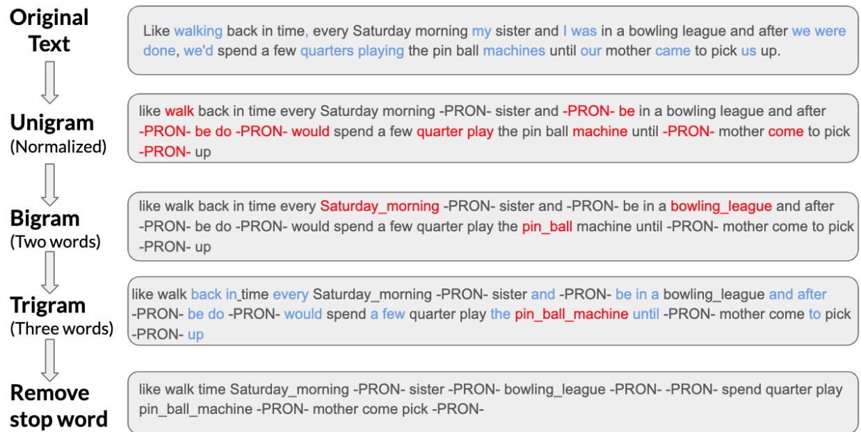
Figure 4.2.1: Example workflow of text normalization, N-gram model and cleaning
