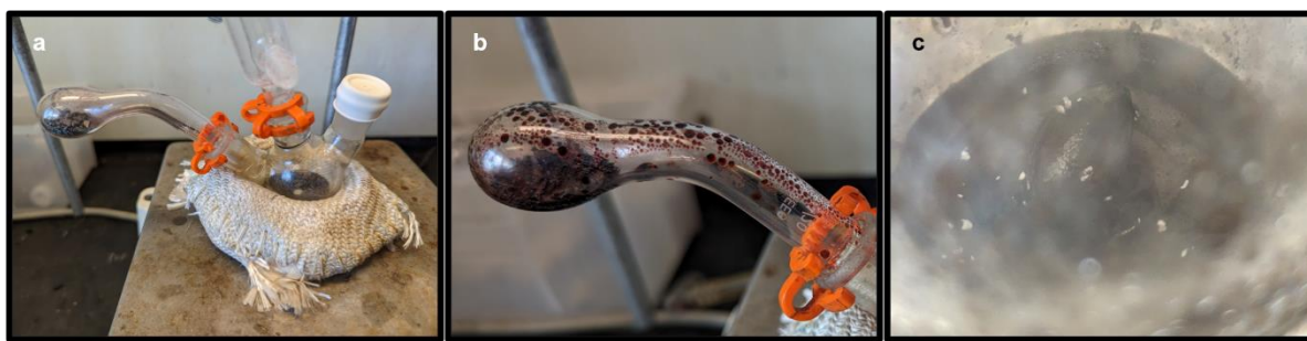
Figure S3. 7. Photographs of different stages of the oxidation-with- \text{I}_2 experiment. (a) The initial physical separation between the nanocrystal toluene suspension in the round-bottom flask and the iodine solid in the Merlic adapter. (b) Red co-condensate droplets of toluene and iodine in the Merlic adapter observed at intermediate times. (c) White copper iodide ( \text{CuI} ) solids spotting the nanocrystal film which formed after evacuating the flask at the end of the oxidation.
