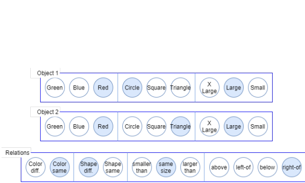
Figure 4: The base scene description of our example represented by memory nodes, encoding “a large red triangle right of a large red circle; having same size, having same color, having different shape”.
