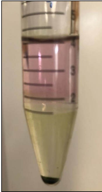
Figure 3-18: The appearance of the Ficoll density gradient as described above, at \frac{1}{4} scale in a 15mL tube after centrifugation at 3,000g for 15 minutes. It remains unclear why this phenomenon involving separation of colors occurred two times only.
