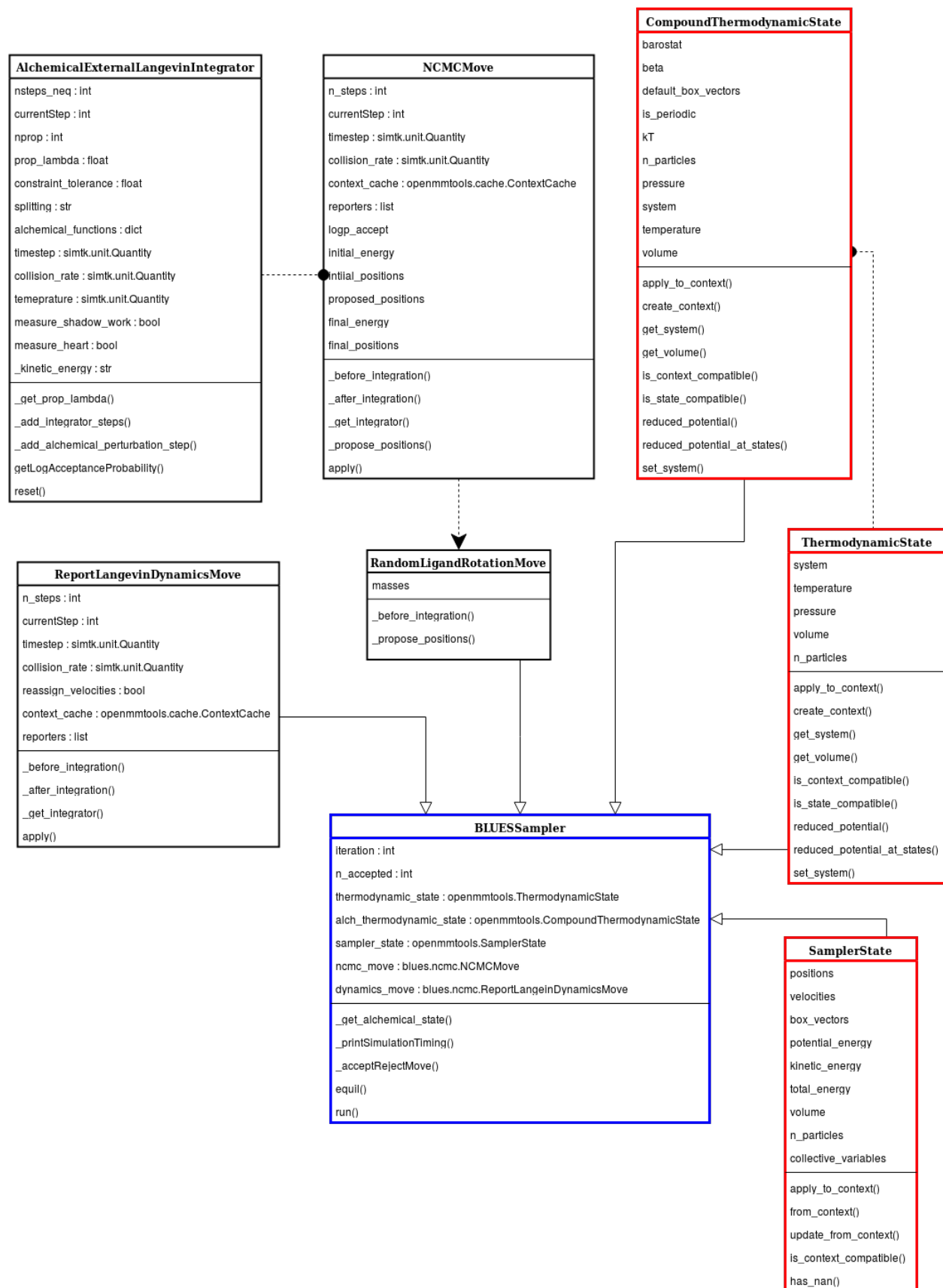
Figure 3.1: BLUES UML Diagram provides an overview of the class objects involved in the BLUES protocol. Each class object is detailed with the attributes and methods belonging to each object.
