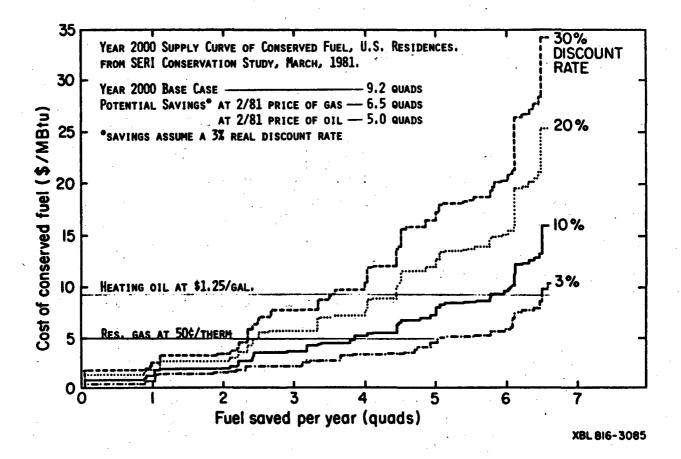
Figure 5-6. A supply curve of conserved fuel with different discount rates. Raising the discount rate increases the cost of conserved energy. It also reshuffled the sequence. This is visible at 3.3 quads, where the reordering led to a sharp jump appearing earlier in the 3% and 10% curves than in the 20% curve.
