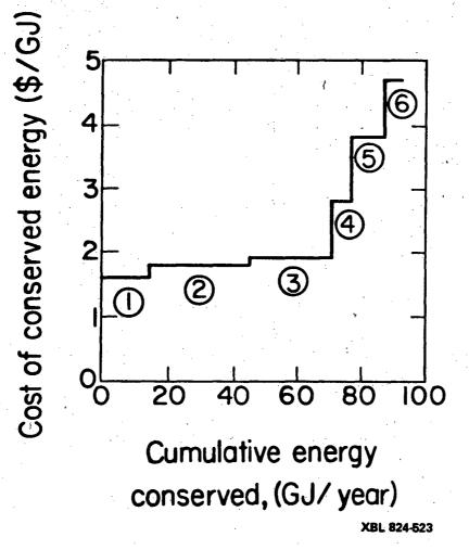
Figure 2-1. A micro supply curve of conserved energy for space heating. See Table 2-2 for assumptions and initial conditions. average energy savings and the number of units to which the measure is applied. This aggregation problem, which one hopes does not introduce large errors, is discussed further in Chapter 5.
