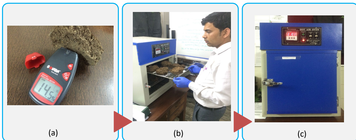
Figure 2.3ab&c: Moisture measurements: (a) moisture meter with sample, (b) sample arrangement in convection oven, (c) convection oven.
