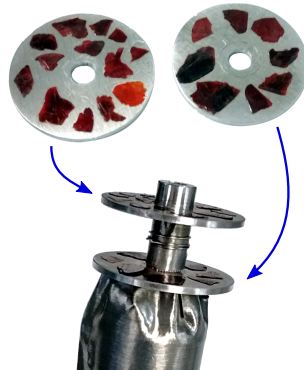
Figure 4.15: \text{KYbSe}_2 sample used to measure the low-energy spin excitations on CNCS. 20 crystals were coaligned and glued to two aluminum plates (top) which were then screwed to a copper rod (bottom). The different crystals are different shades of red because of their different thicknesses.
