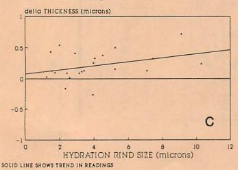
Figure 2 delta-T VS. Rind Thickness
