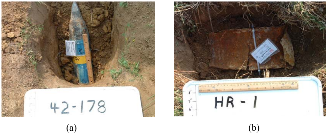
Figure 11. Photos of (a) 4.2" mortar, and (b) a half-round.
