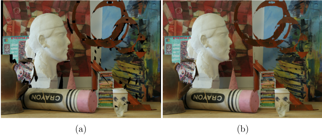
Figure 3.7: Background layer (a) with mapped holes from foreground views (b) after holes are filled.
