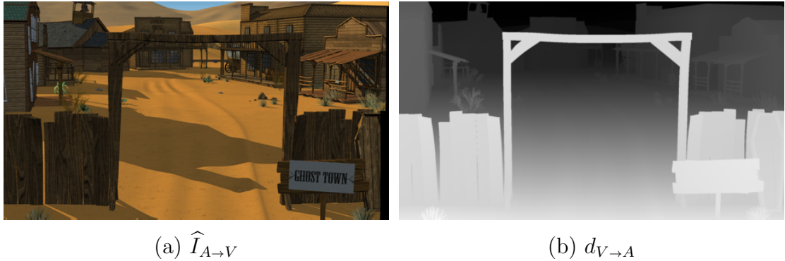
Figure 2.3: (a) Sample rendered image using R-DIBR and (b) the corresponding disparity map for the reverse mapping operation for GTFLy sequence frame #150.
