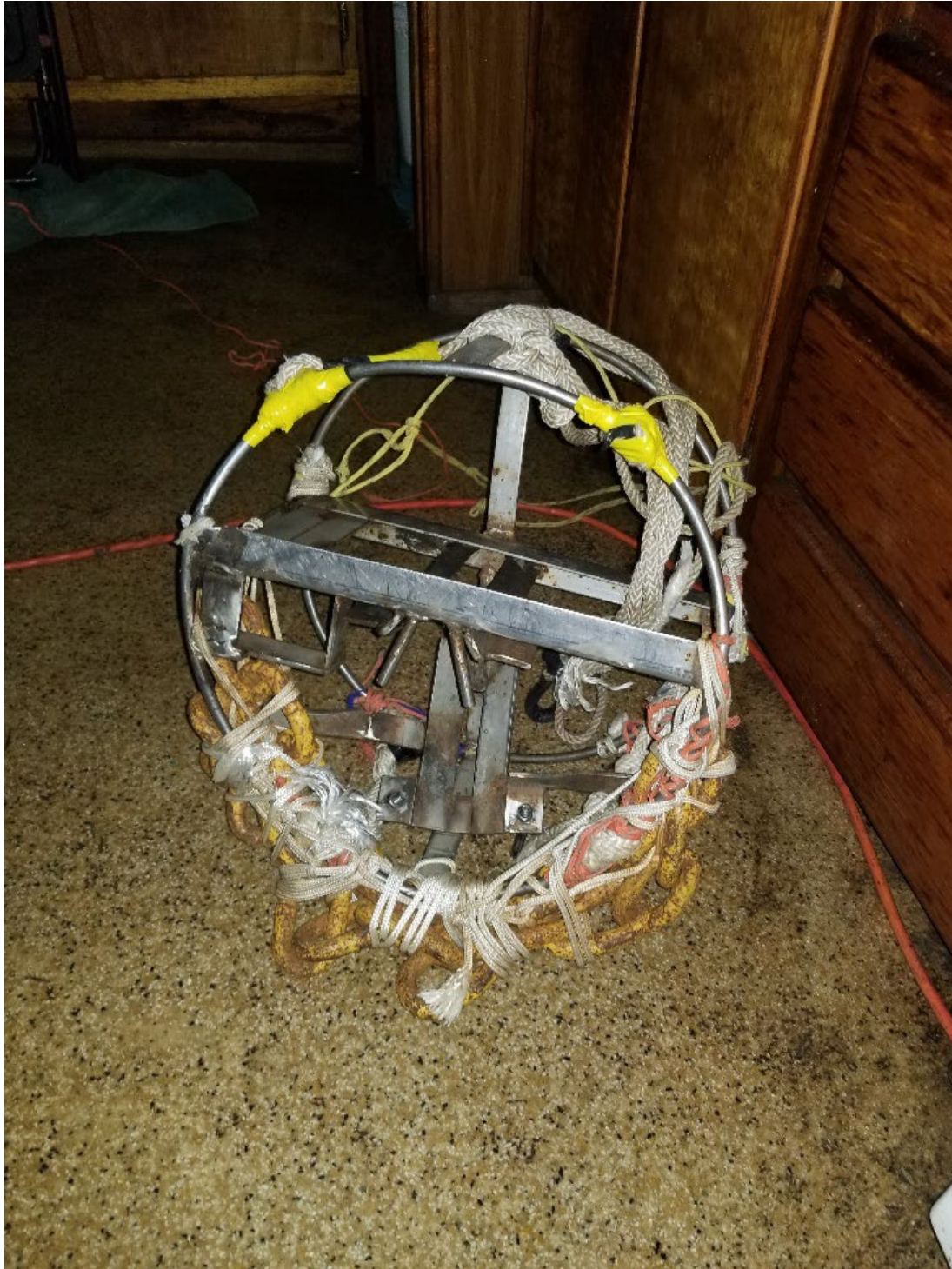
Figure 5.3 A fisherman's research equipment. This was welded together and made for mounting a Go Pro in front and above his trawl so that he could get a better perspective on what is happening in his net when he fishes.
