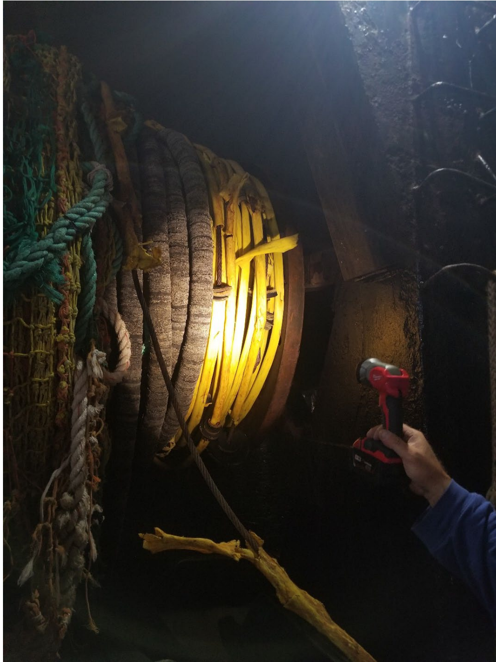
Figure 5.5 Fisherman showing me the modification to the footrope. We are standing at the stern of the vessel.
