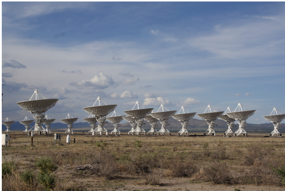
Figure 3.4 The Jansky Very Large Array, located in Plains of San Agustin fifty miles west of Socorro, New Mexico.. There are 27 \times 25\text{m} dishes and have receivers that observe within the centimeter regime. Credit: Katherine Alatalo
