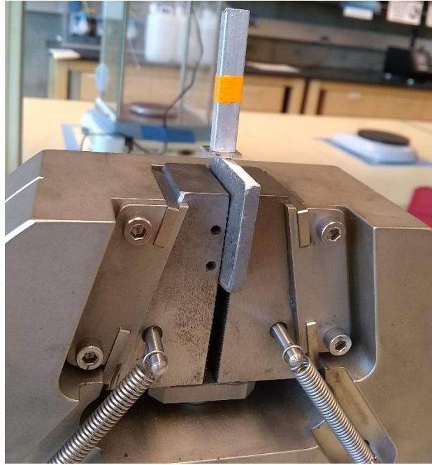
Figure 4.8: Photograph of the direct pull adhesion test setup used for SAA-coated Mg.
