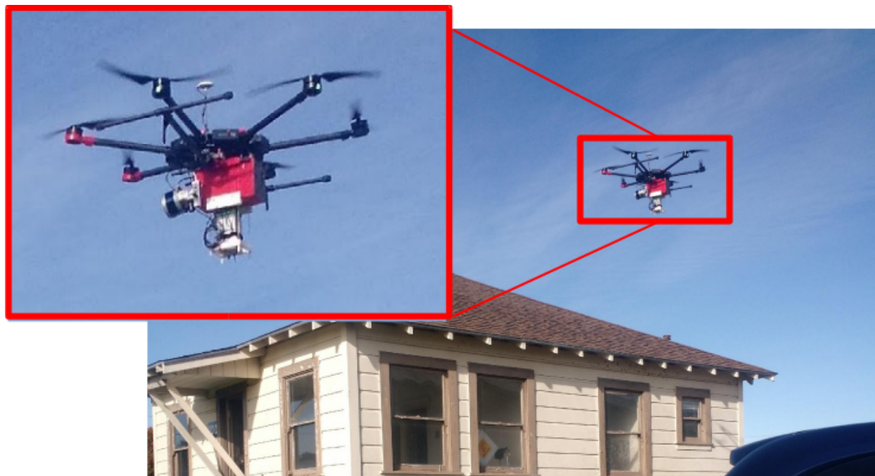
Figure 5.8: LAMP system attached to the UAS. Data collection in this version has minimal feedback provided by the flight controller which can show a HDMI feed of current parameters.
