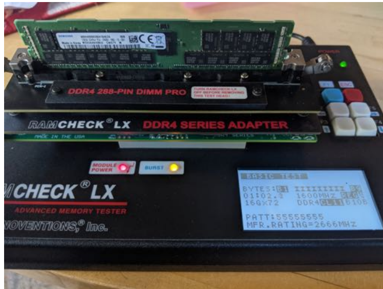
Figure B.6: Innoventions Ramcheck LX Memory Test Platform.
