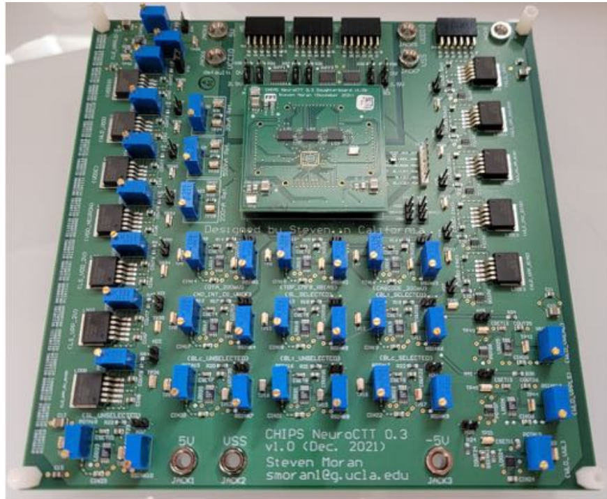
Figure 3.40: Fabricated NeuroCTT 0.3 Mainboard with Mezzanine Card.
