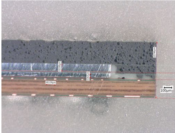
Figure B.4: Cross Section of 2-Layer (2H) Samsung 3DS Memory Devices. Stacked memory devices consist of similar 8Gb DRAM dies. Therefore, 2H and 4H stacked-DRAM devices consist of 16Gb and 13Gb, respectively.
