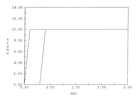
Figure 4: Uniaxial test: loading-unloading.  $\beta=0,\delta/2G\in\{0,\frac{1}{2},1,10\},H=0$
