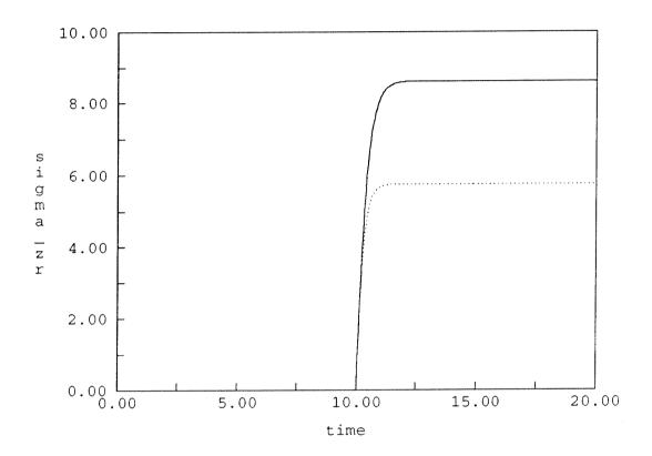
Figure 16: Thin walled tube in tension and torsion (displacement control). Tangential stress  $\tau_{z\theta}$  versus time. For comparison, the solution from the classical model is also presented with a dotted line.
