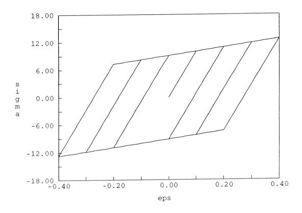
Figure 11: Uniaxial test: cyclic loading. Classical solution.
