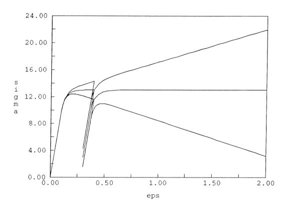
Figure 2: Uniaxial test: loading-unloading.  $\beta=3$  ,  $\delta=G$  ,  $H\in\{-5,0,5\}$
