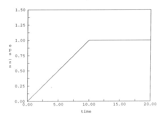
Figure 13: Thin walled tube in tension and torsion (displacement control). Load history in terms of the axial strain  $\epsilon_{zz}$ .
