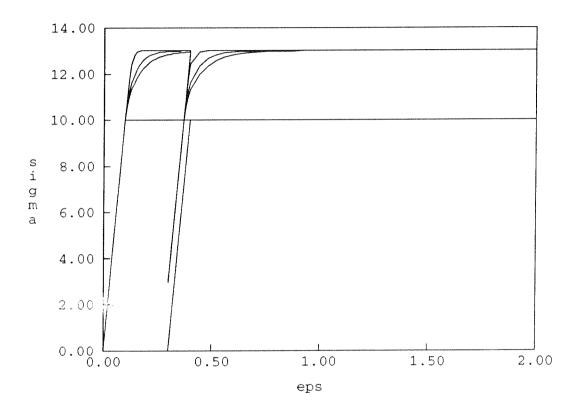
Figure 3: Uniaxial test: loading-unloading.  $\beta=3,\delta/2G\in\{0,\frac{1}{2},1,10\},H=0$
