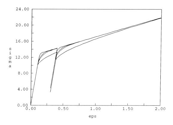
Figure 6: Uniaxial test: loading-unloading.  $\beta=3,\delta/2G\in\{0,\frac{1}{2},1,10\},H=5$
