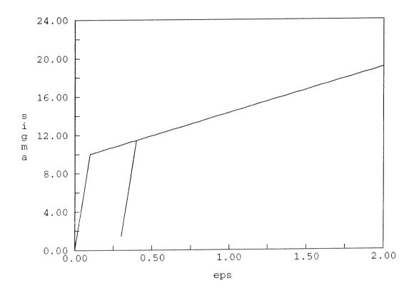
Figure 5: Uniaxial test: loading-unloading.  $\beta=0, \delta/2G \in \{0,\frac{1}{2},1,10\}, H=5$
