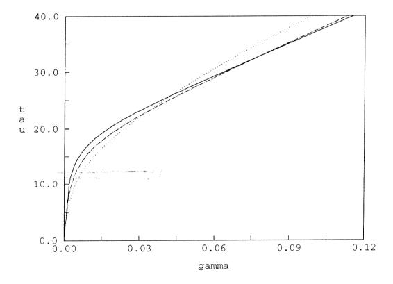
Figure 21: Thin walled tube in tension and torsion (stress control). Tangential stress  $\sigma_{z\theta}$  versus tangential strain  $\gamma_{z\theta}$  for  $\bar{\sigma} \in \{0, 16, 32\}$
