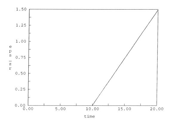
Figure 14: Thin walled tube in tension and torsion (displacement control). Load history in terms of the tangential strain  $\gamma_{z\theta}$ .
