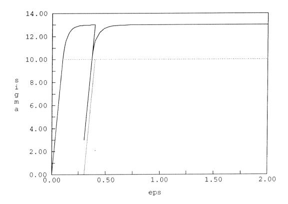
Figure 1: Uniaxial test: loading-unloading.  $\beta=3$ ,  $\delta=G$ , H=0. For comparison, the solution from the classical model is also presented with a dotted line.
