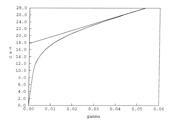
Figure 18: Thin walled tube in tension and torsion (stress control). Tangential stress  $\sigma_{z\theta}$  versus tangential strain  $\gamma_{z\theta}$  for  $\bar{\sigma}=0$
