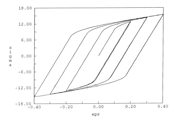
Figure 9: Uniaxial test: cyclic loading.  $\beta=3, \delta=G, H=10$
