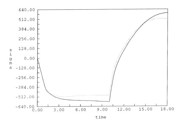
Figure 12: Thick walled tube under pressure. Radial stress versus time. For comparison, the solution from the classical model is also presented with a dotted line.
