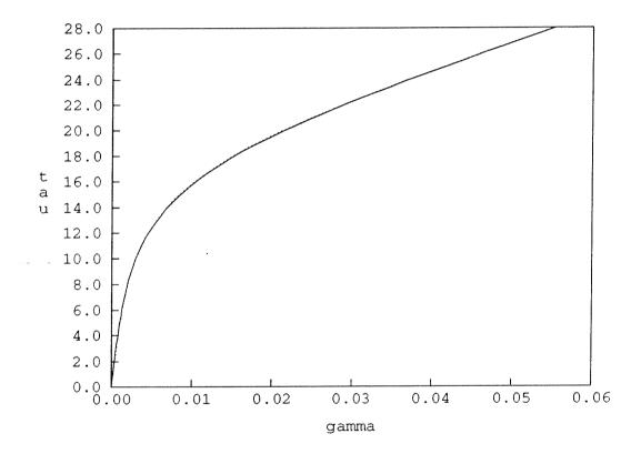
Figure 19: Thin walled tube in tension and torsion (stress control). Tangential stress  $\sigma_{z\theta}$  versus tangential strain  $\gamma_{z\theta}$  for  $\bar{\sigma}=16$
