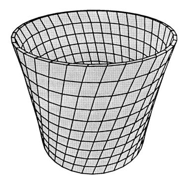
Figure 17: Thin walled tube in tension and torsion (displacement control). Three dimensional mesh at the end of the analysis.
