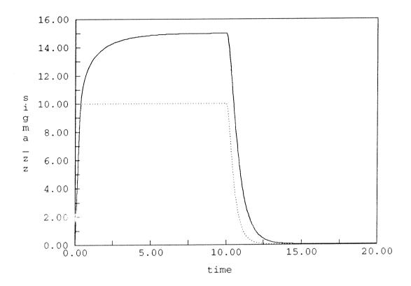
Figure 15: Thin walled tube in tension and torsion (displacement control). Normal stress  $\sigma_{zz}$  versus time. For comparison, the solution from the classical model is also presented with a dotted line.
