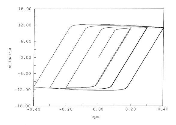
Figure 10: Uniaxial test: cyclic loading.  $\beta=3, \delta=G, H=-5$
