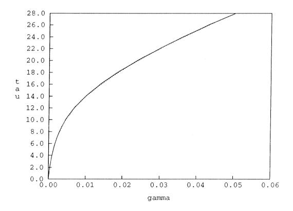
Figure 20: Thin walled tube in tension and torsion (stress control). Tangential stress  $\sigma_{z\theta}$  versus tangential strain  $\gamma_{z\theta}$  for  $\bar{\sigma}=32$
