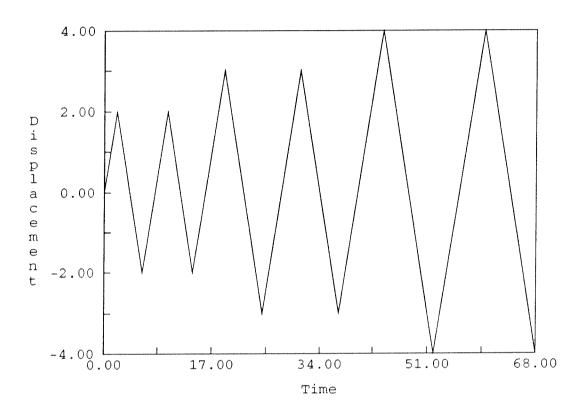
Figure 8: Uniaxial test: cyclic loading. Time history.
