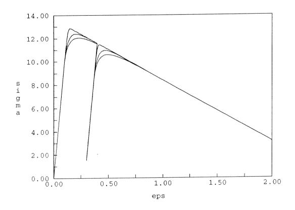
Figure 7: Uniaxial test: loading-unloading.  $\beta=3,\delta/2G\in\{\frac{1}{2},1,10\},H=-5$
