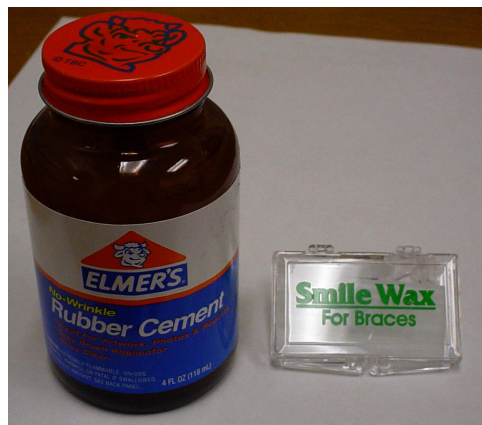
Figure 3. Rubber cement and was for mounting capillary to the post.
