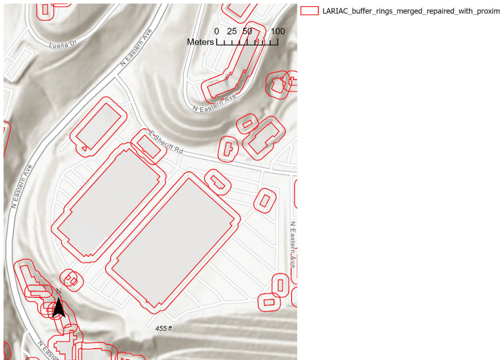
Figure A-10. Excerpt from buffer-ring feature class showing 10-m-wide buffer rings drawn around buildings.
