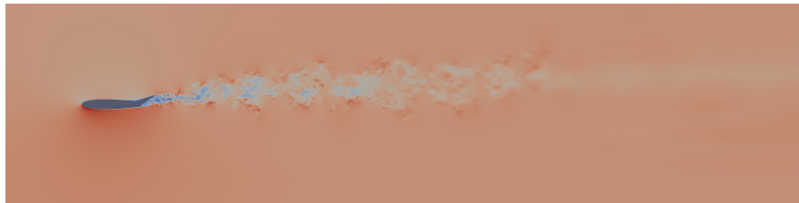
Fig. 8: From a 1M-way parallel PHASTA run on mi ra at Argonne National Laboratory, this image is a zoomed-in view of a 2D slice from 3D volume. This numerical simulation models the flow over a vertical tail-rudder assembly for a geometry that exactly matches the configuration of an ongoing wind tunnel experiment. Image courtesy K. Jensen, A. Bauer, A. Ayachit, and P. O’Leary [1].
