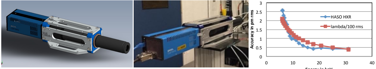
Figure 11. LEFT, rendering of the optimized HXR wavefront sensor at Imagine Optic SA . CENTER, The WFS installed at the APS 7-ID beamline. RIGHT, Calculated accuracy of the wavefront sensor, compared with a \lambda/100 value.
