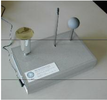
Figure 3. Indoor Comfort Monitor used in Operable Windows field study.
