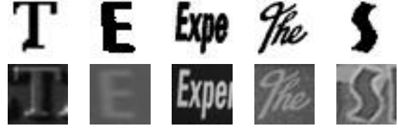
Figure 2. Some resized binary patches fed to CNN, together with their original grayscale counterpart. Note the presence of a trigram and of a four-gram.
