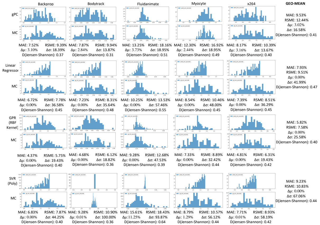
Figure 4.5: Comparing gPC estimators and theoretical limits of linear regressor, support vector regressor and gaussian process regressor. gPC models are still trained with merely 10 samples while all other regressors are trained with the exact test set, i.e., 100 Monte-Carlo samples, which should work in their favorite and serve as an upper bound of how well these regressors can perform on this test set.
