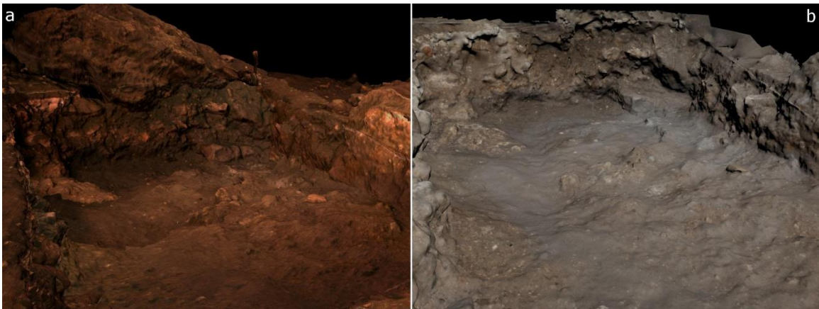
Figure 45. Three dimensional texturized models of Unit 1, Level 6 (cave entrance chamber), acquired using two different techniques (TLS and DSM): a. TLS; b. DSM.
