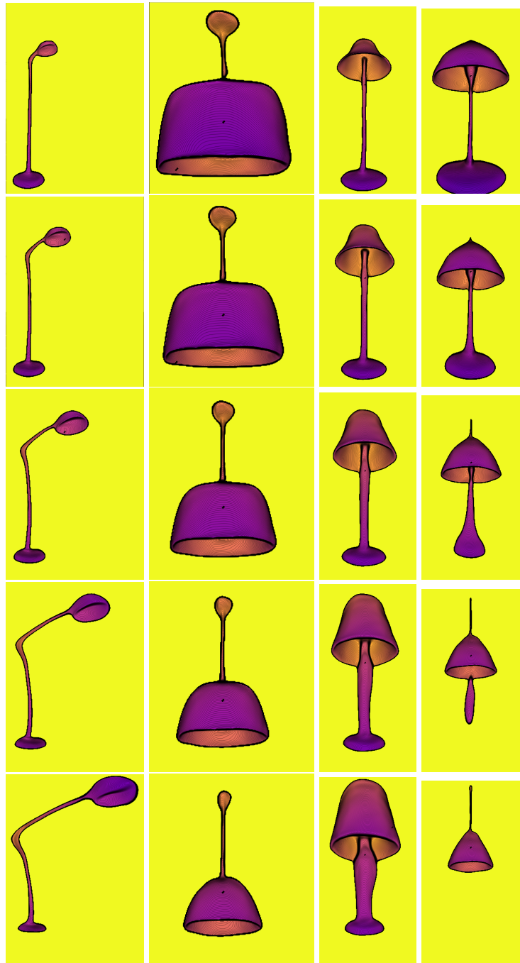
Figure 3.14. SDDF shape interpolation between two lamp instances. The first and last row show the SDDF output from the same view for two different instances from the training set. The rows in the middle are generated by using a weighted average of the latent codes of the upper-most and down-most instances as an input to the DeepSDDF network. In each column, from top to bottom, the latent code weights with respect to the upper-most instance are 1, 0.75, 0.5, 0.25, 0, respectively.
