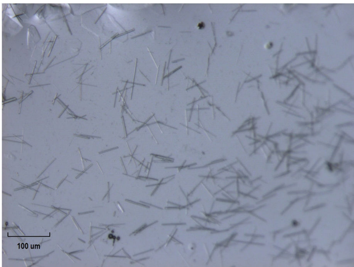
Fig. 7. Optical microscope image of IPNS • Fe • ACV microcrystals.
